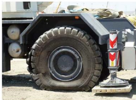
Ruptured Tyres and Shattered Cab Window
